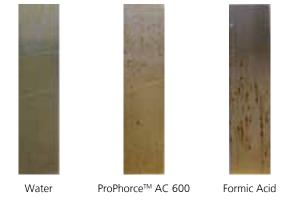
Corrosivity of ProPhorce<sup>™</sup> AC 600 on steel strips submerged in the liquid, measured as weight loss.
